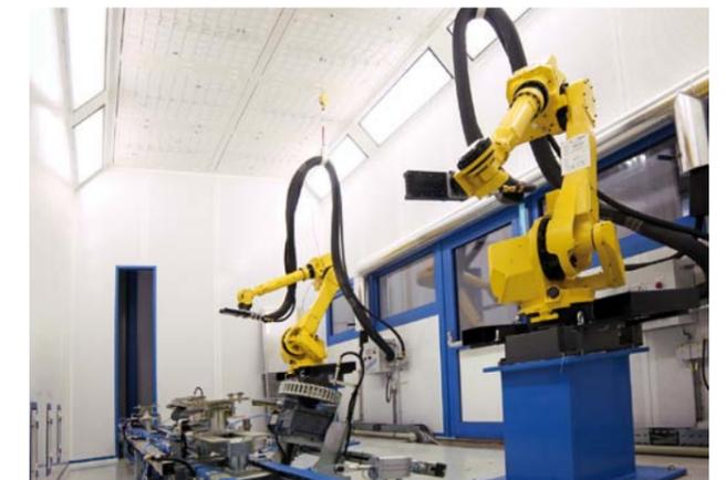
includes air handling systems with humidification and cooling functionalities. Coating booths with water separation of excess coating materials are used for this line in order to maintain stable conditions during coating operations.
