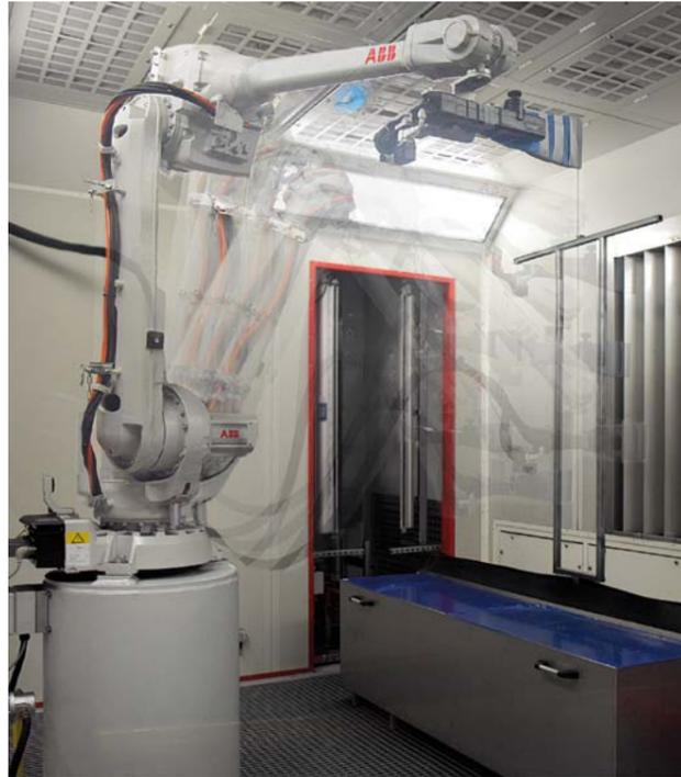
of automatic coating systems in terms of scope as well as the high technological standard of the line. The coating line is designed for comprehensive surface finishing of metal and plastic parts. Parts are pre-treated by flaming and dry ice blasting. Liquid coating materials are applied in two coating booths with water filters. Design of individual process sections of the line allows application of advanced coating systems, such as high-gloss finish.
