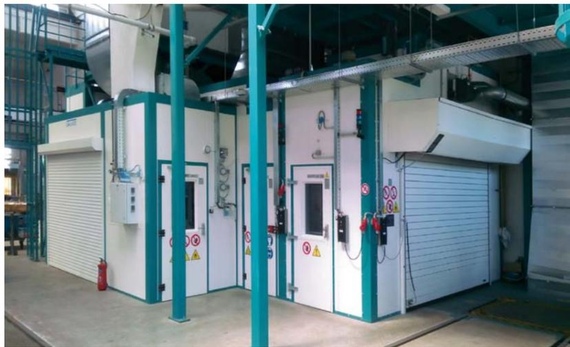
The line is fully automatic. Its core consists of a five-chamber pass-through zinc phosphate spraying machine followed by blowing, drying and cooling operations. The coating section of the line consists of two coating booths at two different elevations, followed by volatilization and drying operations.
